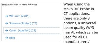
models) and 2 specific options for the Siemens Straton, and Canon Aquilion systems, as they have specific X-ray spectra profiles.
